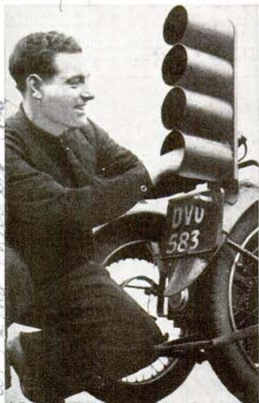
Special shades are fitted over the rear lights of motorcycles used to lead buses and streetcars in Manchester, England, in fog or blackout
